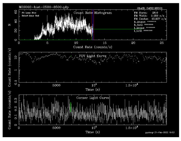
In the plots above, it can be seen that either the entire data or most of the data is flared. Thus, the cleaned events list would have a very low number of count rates, which can be verified by creating an image of the observation.
