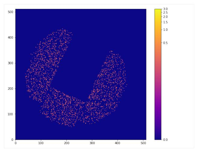
Here, it can be seen that there's hardly an image and only a few pixels, which indicate the low number of count rates in the cleaned events list.
