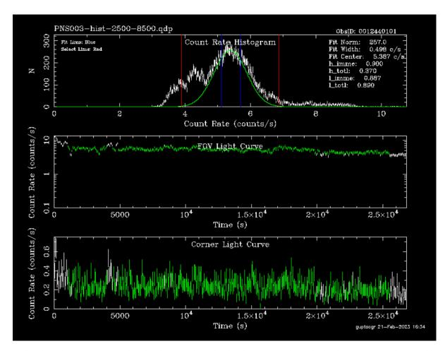
In the plots above, we can see that the cleaning algorithm has been correctly applied. The count rates above and below those determined by the Gaussian (in the histogram) have been removed/cleaned from the data. These removed count rates are displayed in white. All the remaining count rates are displayed in green, which are to be used in the cleaned events lists to obtain an image of the observation.
